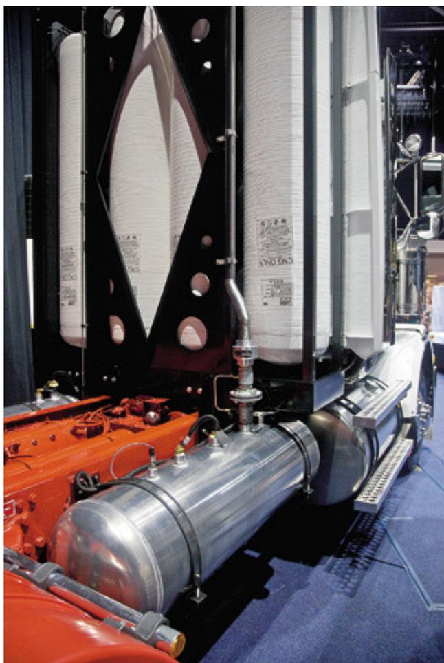
Normal CNG engines use the gas at a much lower pressure than LNG engines. With CNG, the gas is vented into the combustion chamber at relatively low pressures and is ignited using spark ignition. This requires a completely different kind of engine, specifically designed for use with CNG. The Westport alternative uses tried and trusted diesel technology and adds on a different kind of fuel injection system, no other changes are made to the ISX.
